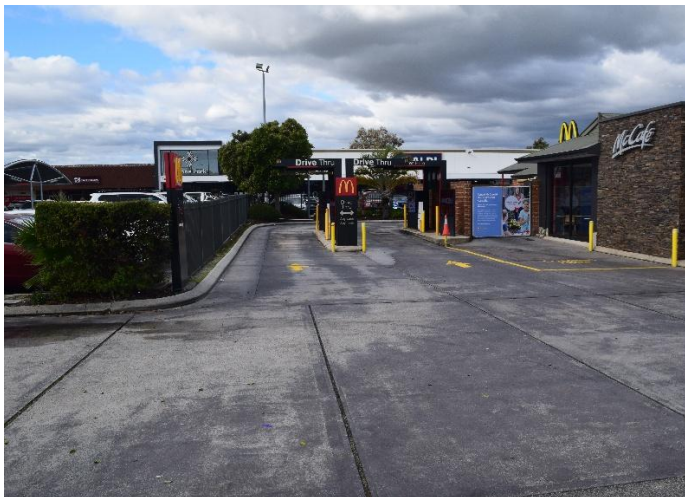
Figure 3: Good Natural Access Control to guide vehicles through a drive-through service zone and use of bollards, colour and signage are further contributors indicating that this area is for vehicles only and not for pedestrian access.
