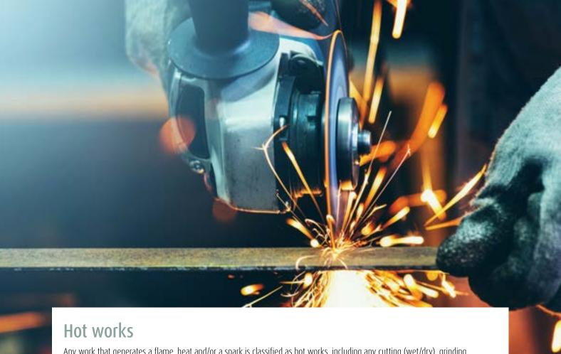
Any work that generates a flame, heat and/or a spark is classified as hot works, including any cutting (wet/dry), grinding, welding and the use of an open flame.
