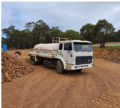
Plate 4-1: On site dust management actions including the use and presence of a water cart
