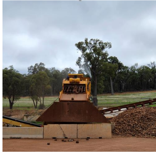
Plate 4-2: On site dust management actions including use of a sprinkler system during processing.
