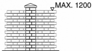
FLEMISH OR ENGLISH BOND BRICK FENCE (USED WITH EARLIEST HOUSES) FOR CONSERVING OLDER HOUSES
