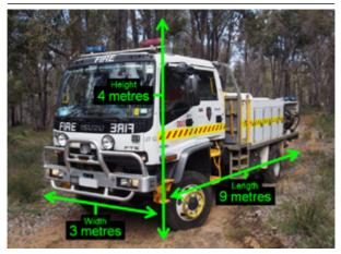
Firebreaks, including corners, must be constructed to accomodate this vehicle
