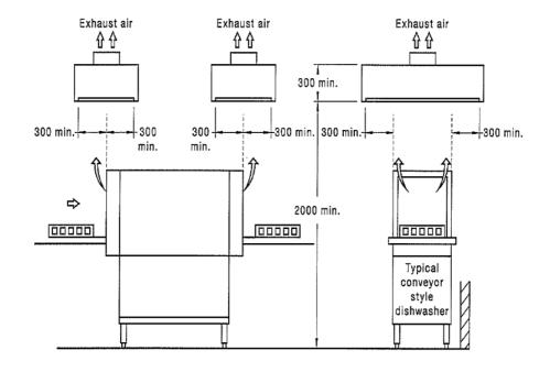
FIGURE E10 TYPICAL CONVEYOR DISHWASHER STYLE HOOD TYPE 6 CANOPY
